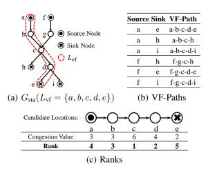
Fig. 6: An example for ranking repair locations.
